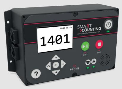
The new and robust **Edge Intelligence (EI) Platform** on which the smaRt Counting software runs allows to permanently install the hardware directly in the barn or to move it from one barn to the other, if required. The Ro-Main EI Platform is the world's first edge computing hardware that makes artificial vision possible in the extreme conditions of an animal barn (IP67).
